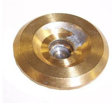
Concave side of Spring Plate
