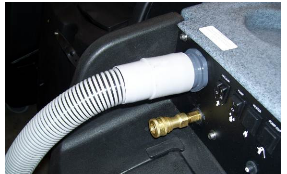
VACUUM CONNECTION WITH STANDARD BARB AND VINYL CUFF
